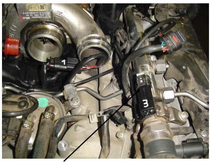
This connector must be disconnected from the right side flap rod sensor of the intake manifold valves after testing device installation. Instead, this connector connects to the third testing device connector. Itself right side of the flap rod sensor remains disconnected.
