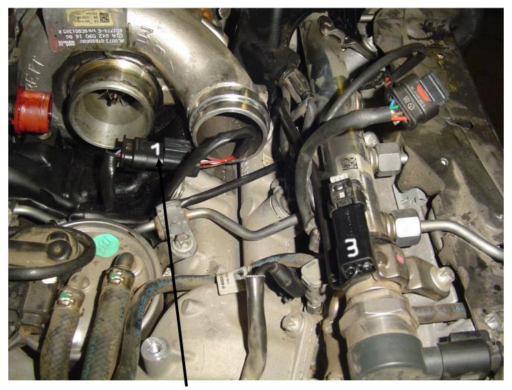
This connector must be disconnected from the control engine of the intake manifold after testing device installation. Instead, this connector connects to the first testing device connection.
